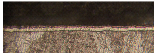
Figure 3. The functional intermetallic-ceramic IMCER (x460).
